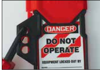
Loop end brace and secure in place by padlock
